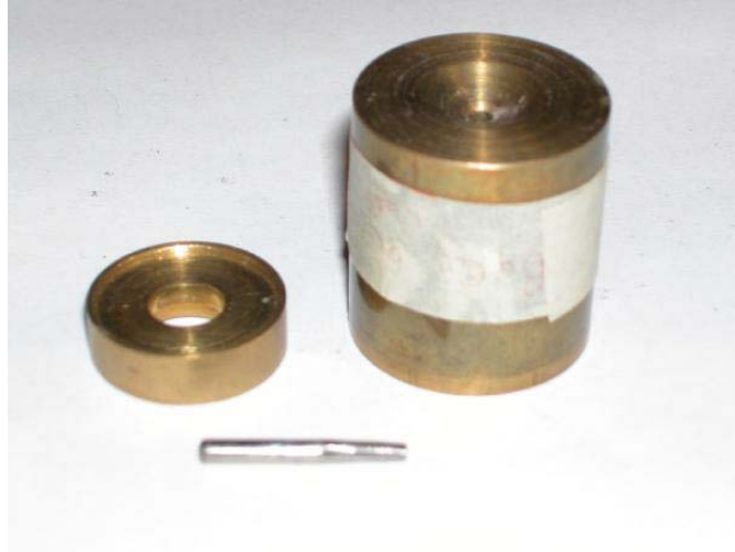
Figure 1.3: Picture of the jig (made by C. Looney) for removing the backing from the CuBe backing plate. The backing plate is placed upside down on the disc on the left, and the cylinder on the right is placed over the top. The dowel in the foreground is placed through the hole in the top of the cylinder and is used to press out the backing, with help of the hydraulic press. If using the backing pieces with the 15^\circ cone, make sure the appropriate-cone-shaped dowel is used to remove the backing piece so that the force is evenly distributed and the backing piece doesn't break.
