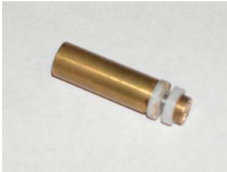
Figure 4.2: The coil form used for winding the side-by-side coil system.
