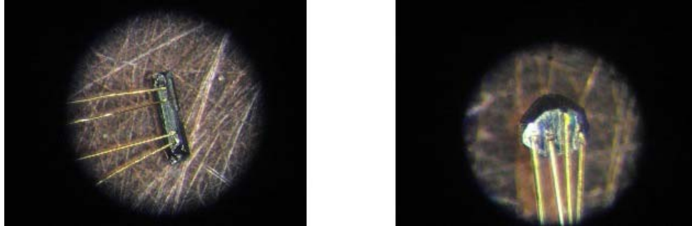
Figure 5.6: Examples of samples wired with the micro spot welding unit. (left) A single crystal of \text{Yb}_2\text{Fe}_{12}\text{P}_7 with length 1 mm. (right) A 370 \mu\text{m} long single crystal of unknown composition grown with U, Fe, and P in a Sn flux.
