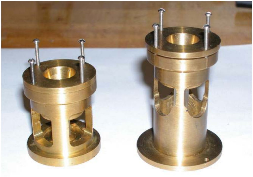
Figure 1.2: Jigs for supporting diamonds during gluing. The cell-body backing plate sits in the jig on the left, while the jig on the right slides over (and can be securely fastened to) the piston.
