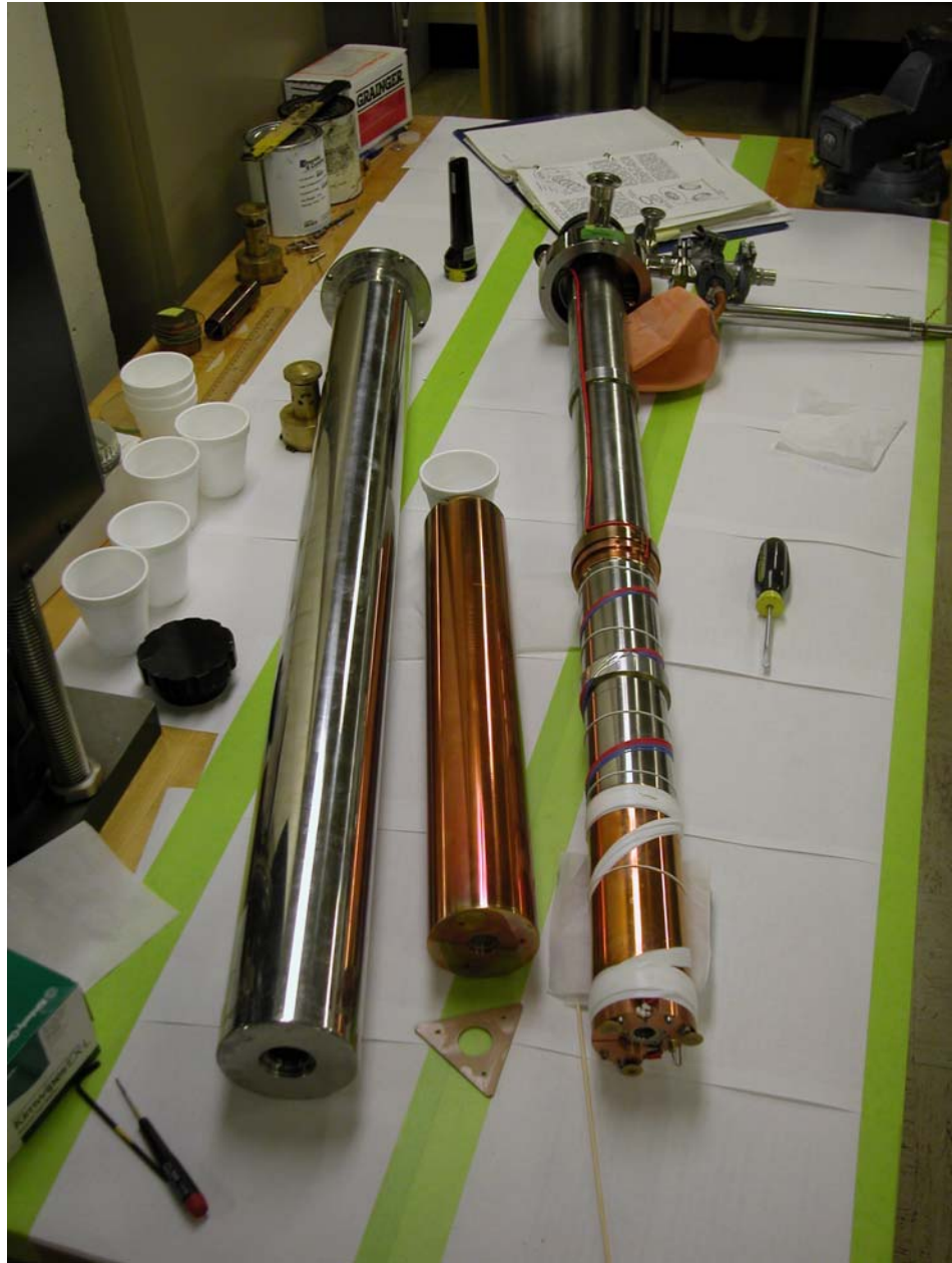
Figure 1.7: Oxford “flow” cryostat. (left) outer case with quartz window; (middle) heat shield with quartz window; (right) sample tube with sapphire window and copper gasket seal. Heater and Rh-Fe thermometer are in holes in two of the three copper blocks on the bottom of the sample tube.
