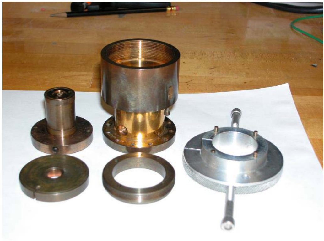
Figure 1.1: The DAC. In addition to the piston and body, the force plate (which sits on top of the diaphragm, not shown), the retaining ring, and the torquing tool for the retaining ring are pictured from left to right in the foreground.
