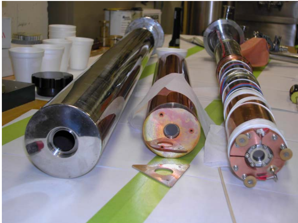
Figure 1.8: Oxford “flow” cryostat. (left) outer case with quartz window; (middle) heat shield with quartz window; (right) sample tube with sapphire window and copper gasket seal. Heater and Rh-Fe thermometer are in holes in two of the three copper blocks on the bottom of the sample tube.
