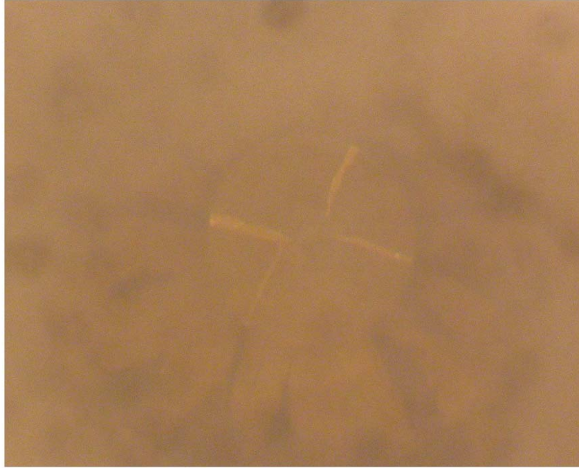
Figure 9.9: Picture taken through the top diamond when it was under pressure.
