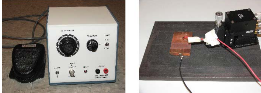
Figure 5.1: (left) Micro spot welding power supply and foot switch. (right) Micromanipulator with magnetic base, mounted on a steel plate. The tungsten wire electrode is taped to the micromanipulator.
