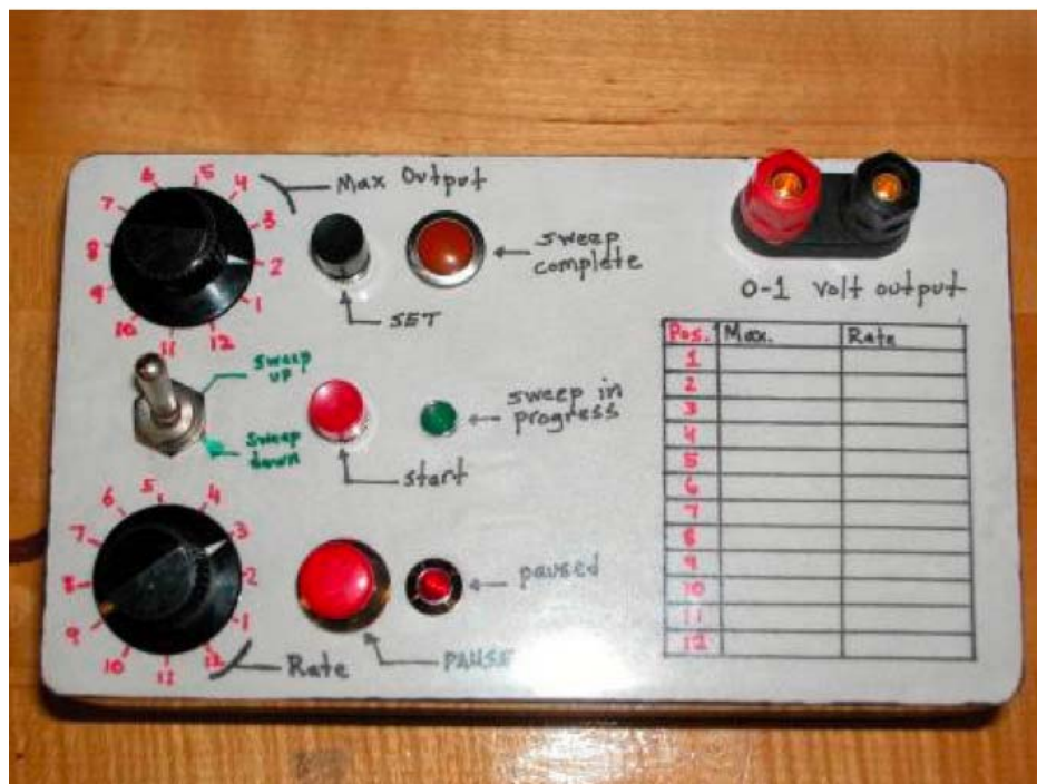
Figure 6.1: Controls for current ramping device
