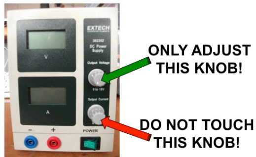
Figure 1: How to use the power supply during lab. Check that the bottom knob is turned all the way up and leave it there.
