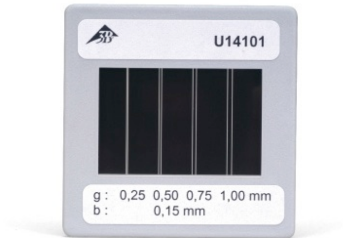
Figure 7: Slide containing four double slit patterns
