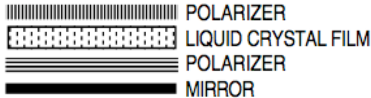
Figure 4: Cross-Sectional Views of an LCD Display on a Calculator
