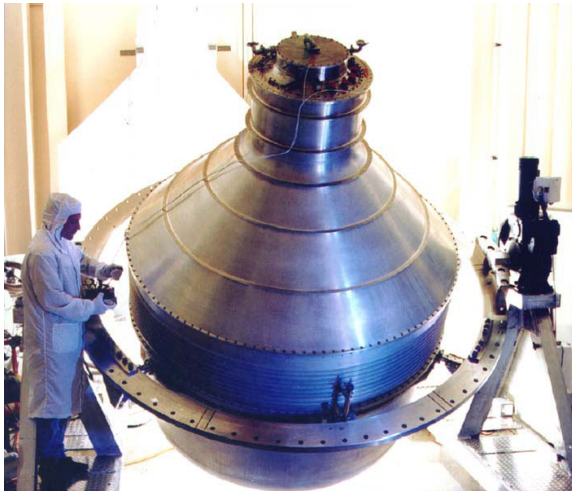
The 645-gallon GP-B flight dewar (liquid helium)
